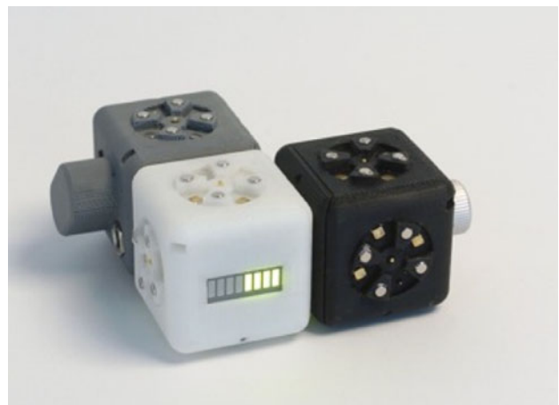
Fig. 2 The simplest robot: a twist sensor block (the black block with a knob on the right) and a bar-graph action block. The gray block in back is a battery block (color figure online)
