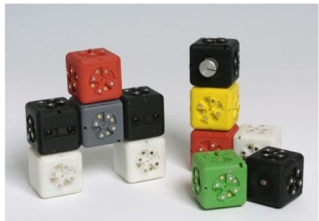
Fig. 1 roBlocks is a heterogeneous modular robot construction kit. The white blocks are 'action' blocks, the black blocks are 'sensor' blocks, and the colored blocks are 'think' or operator blocks. They snap together and transmit power and data through the magnets and spring probes on their faces (color figure online)
