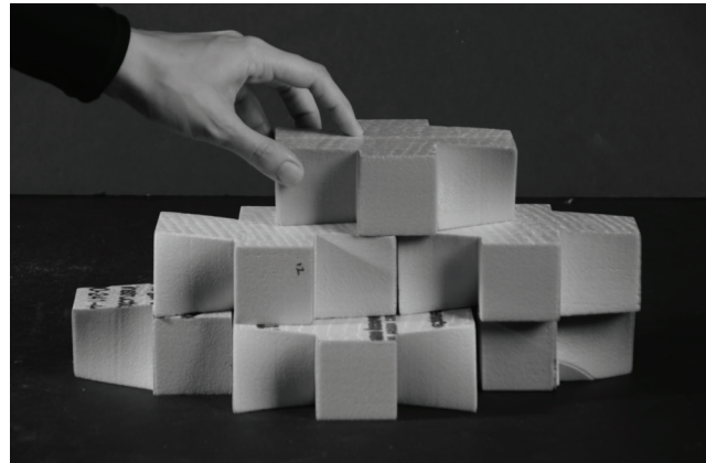
Figure 4. A wall configuration created using the robotically fabricated modules.
