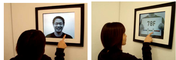
Figure 1. a) RayMatic is a playful interface to a home heating system. b) Adjusting the set-point on the RayMatic.
