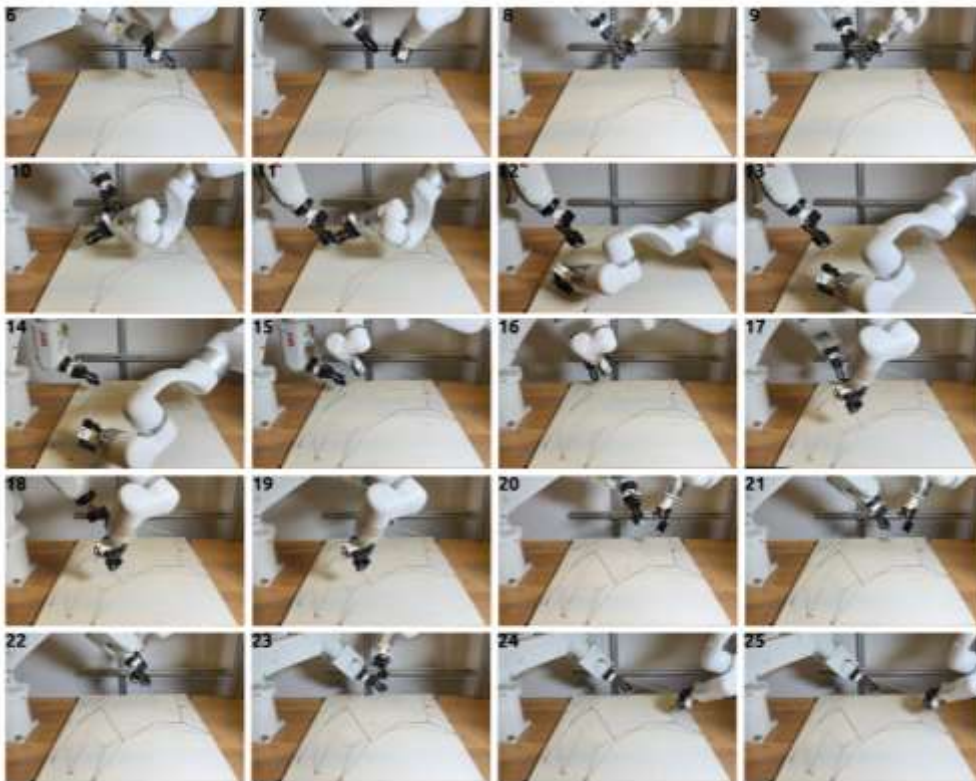
Figure 10: Interpolating robot motions to take rotary roles for placing new components and acting as additional support.
