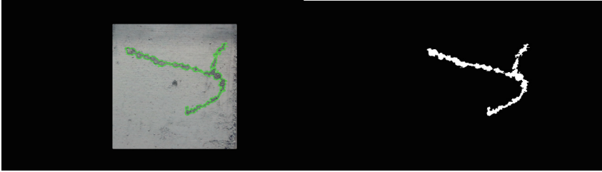
Fig. 8 Detected contours of the printed pathway. Left: Detected contours of the printed pathway. Right: The pixels of the printed part are labeled in white.
