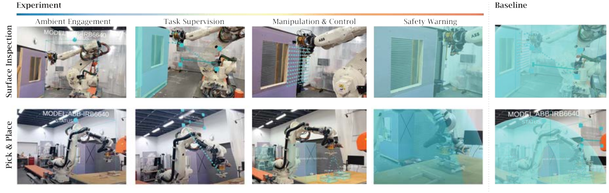
Figure 5.7: Experiment and baseline setup for surface inspection and pick & place scenario, the baseline setup displays all virtual information at the same level of details, the experiment setup selectively displays the relevant virtual information tailored to the current human-robot proxemic level. Image credit: Author.
