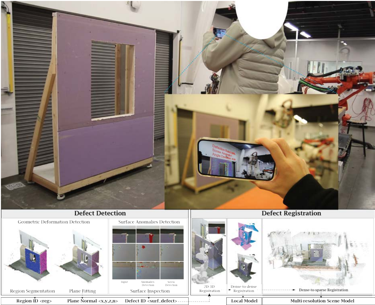
Figure 6.4: The defect detection result is registered to the physical environment and visualized through an AR interface. Image credit: Author.
