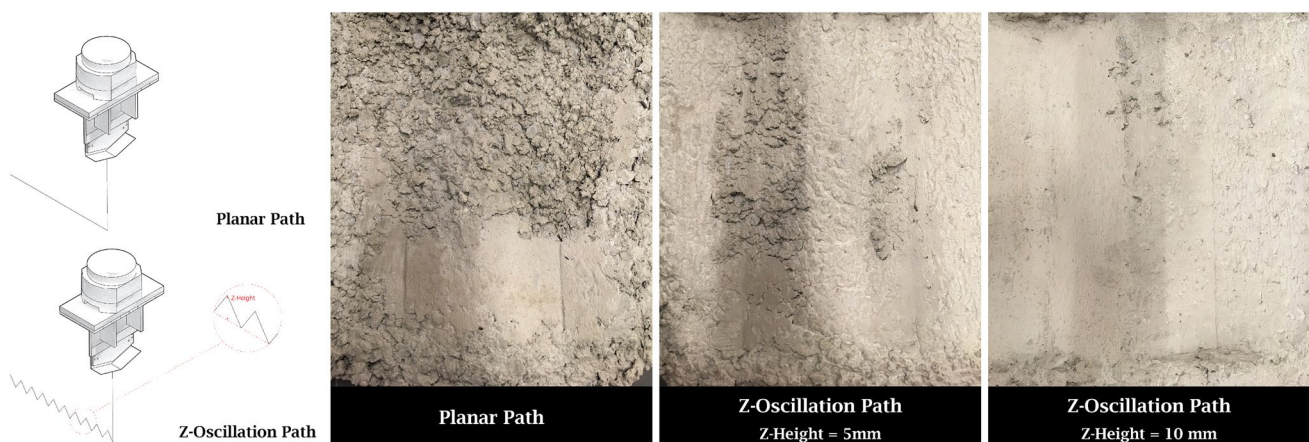
Fig. 9 Adding Z-oscillation into tool path can improve surface quality of concrete panels
