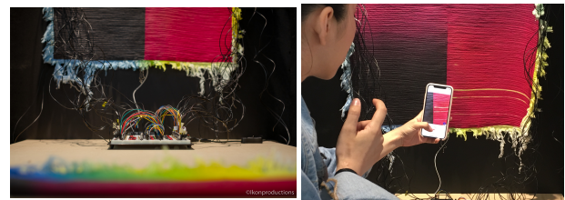
Figure 3: Wanted Design: Fabric Partition with thermochromic pigment and conductive thread. Image Credit: Daniel Rosenberg
