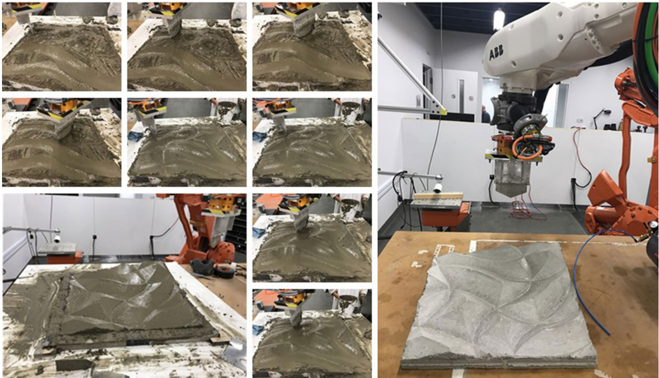
Fig. 12 Tooling process and finished panel demonstrating Profile-3D-Printing
