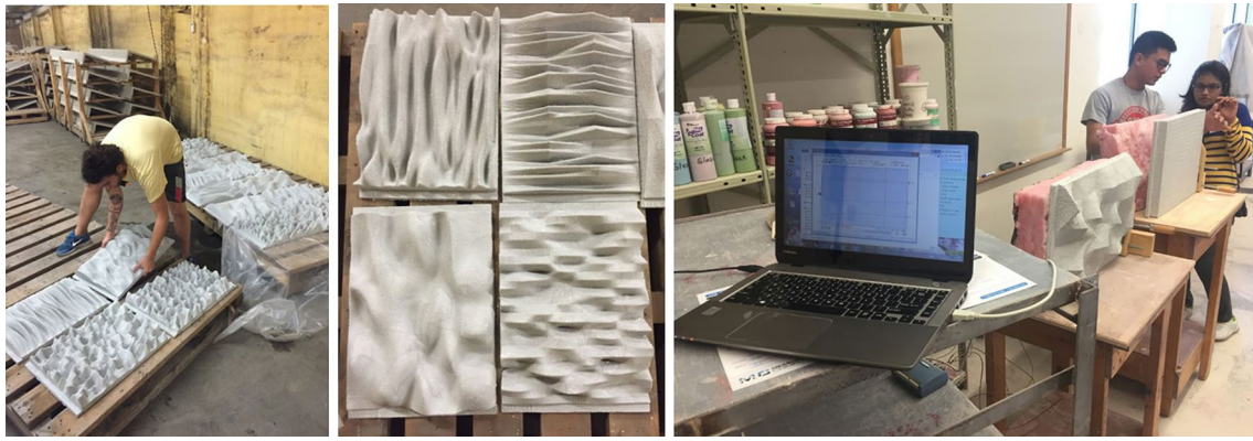
Fig. 1 (Left) Prototyping and (right) thermal testing of mold-cast UHPC panels with complex surface geometry
