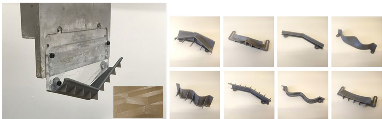
Fig. 10 Examples of interchangeable, custom 3D printed tool heads for rough and finish surfacing of concrete tested by authors with inset of finished pattern
