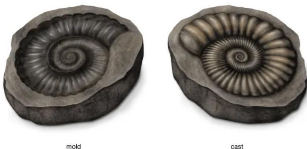
Figure 3.6 Illustration of a positive object vs its negative mold. The mold (left) contains a cavity that is the exact inverse of the desired object (right), so that casting or forming material into the cavity will produce the object. In our case, the negative mold is 3D printed, and the “casting” material is a heated plastic sheet formed into it.
