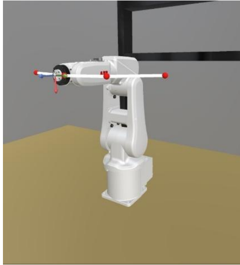
Figure 30: Waypoint visualization showing motion sequence from a left perspective.
