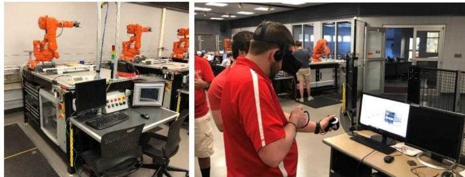
Figure 5: ABB RobotStudio VR test environment with virtual robot work cell.
