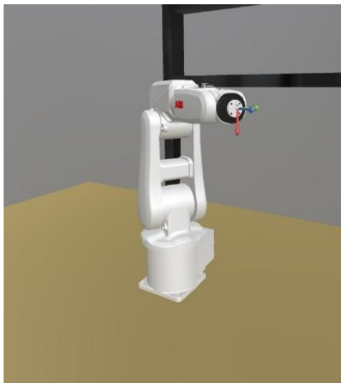
Figure 31: Robot model in default home position before waypoint path execution.
