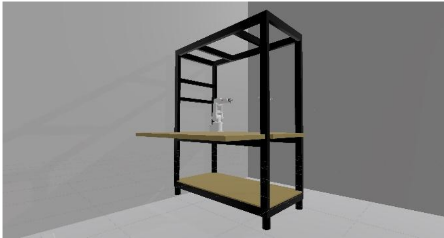
Figure 16: Virtual workstation modeled in Unity based on the physical ABB IRB 120 setup.
