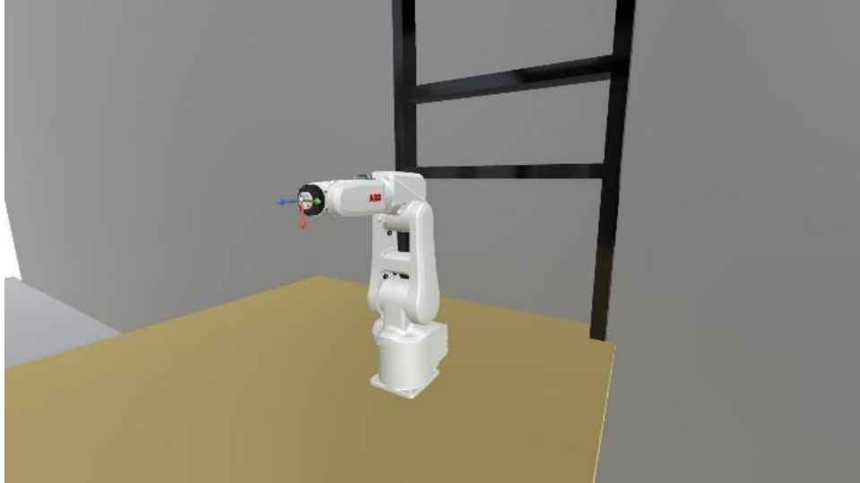
Figure 21: Right-side camera view of the ABB IRB 120 in the virtual dFab Lab.
