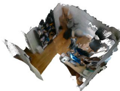
3D mesh reconstructed from RGB-D video using SLAM
