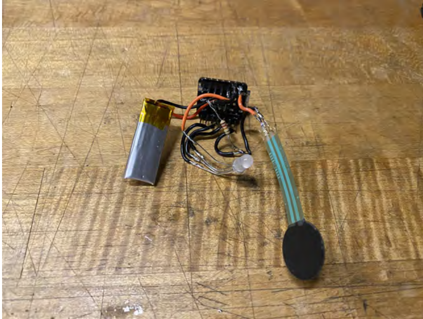
Figure 36: Prototype 01 - The micro control unit inside the squeeze ball
