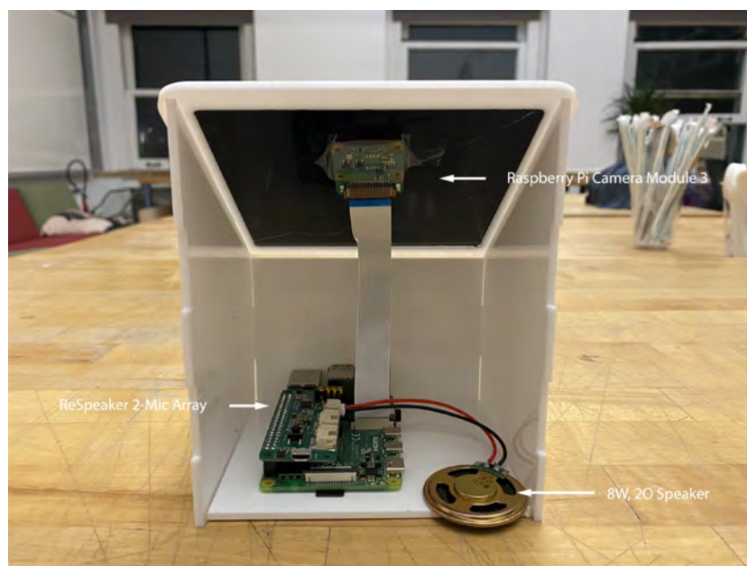
Figure 26: I'm watching: annotated components
