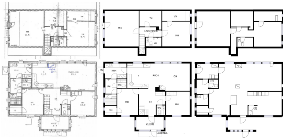
Figure 28. Example result using CubiCasa5k dataset and pipeline provided. (left to right, original floor plan, SVG label, automatic prediction) 90
