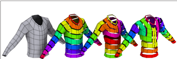
Fig 49. Labeling input meshes into knitting rows [40]
