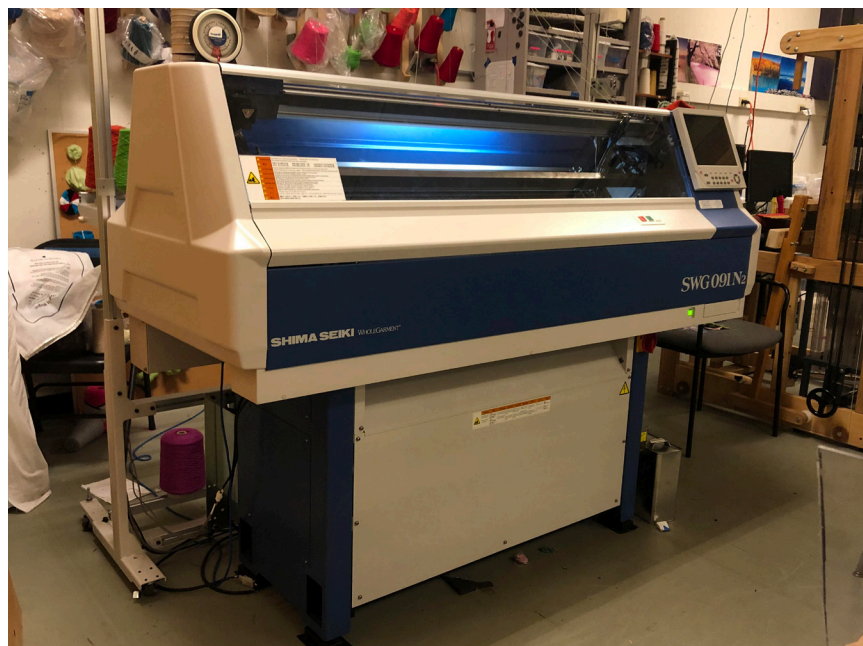
Fig 14. Shima Seiki SWG-X 2-bed flatbed industrial knitting machine
