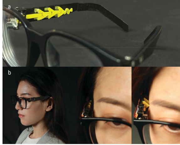
Figure 4-11: (a) A row of 3 tactors integrated into an existing pair of glasses (b) a user wearing a pair of Parametric Haptic-integrated glasses in daily life, the glasses can unobtrusively and effectively deliver information.
