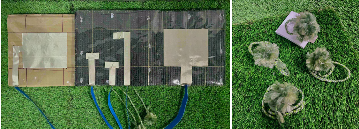
Fig. 38 (left): Backside of the Grass Pad , Fig. 39 (right): Custom capacitive pom-poms.
