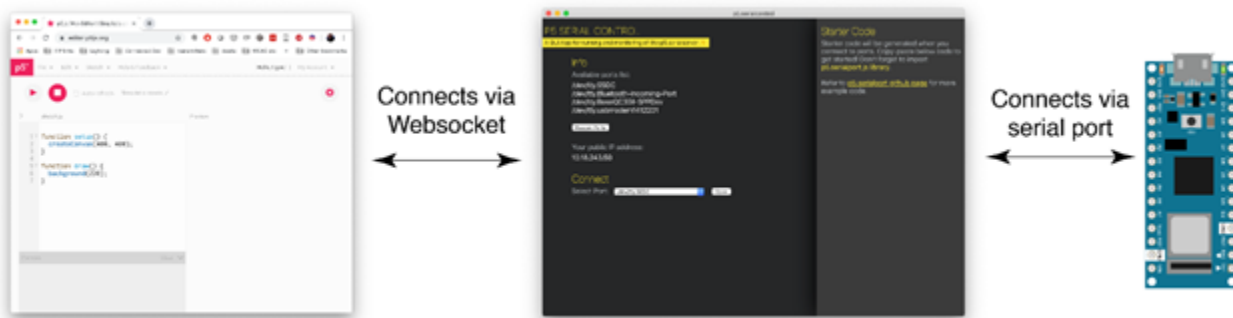
Diagram of the connection from the serial port to p5.js through p5.serialcontrol. Image Credit: ITP Physical Computing.
