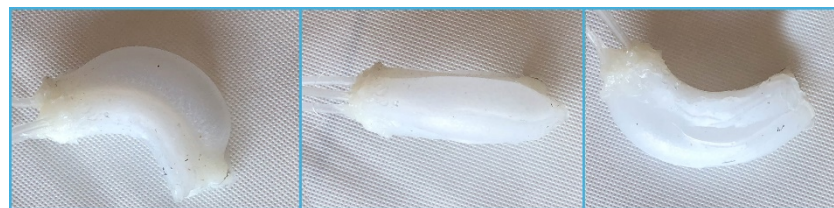
Figure 9. FEA prototype with three distributed air channers
